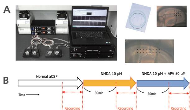
**FIGURE 1:** A, MED64 Quad system (left) and MED Probe 16 with the pictures of hippocampal slices on the probes (two electrode layouts: 4x4 and 2x8) (right). B, experimental workflow for measurement of NMDA treatment in absence or presence of NMDA antagonist APV.
