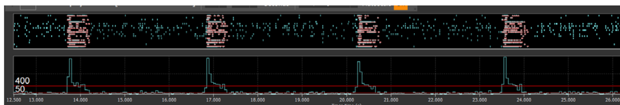
Figure 14. Raster plots (top) and Spike frequency histogram computed (bottom) and displayed in the MEA Symphony.
