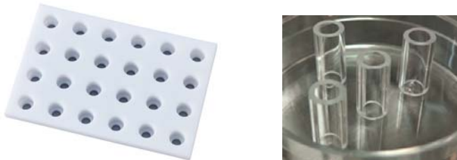
Figure 1. CellSpotter24 eco (left) and cloning rings (right). Cells will be amounted onto the recording electrodes through cloning rings placed in the central hole of the CellSpotter.
