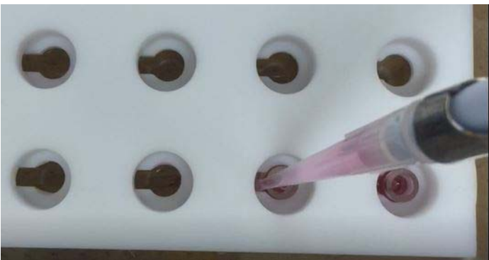
Figure 7. Add the Medium A to the well through one of the side holes.
