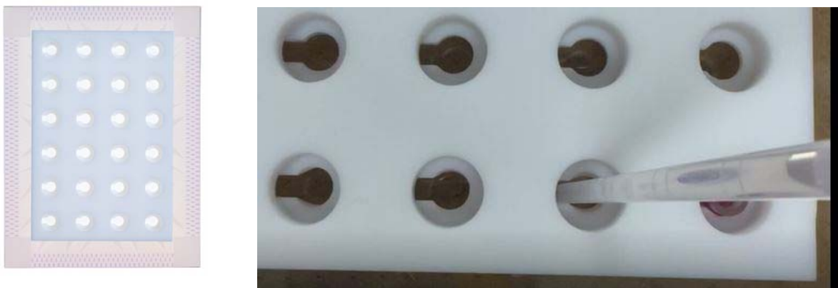
Figure 4. Placing the CellSpotter onto the MEA plate (left) and remove the SureBond from a well through the side-slot (middle, right).
