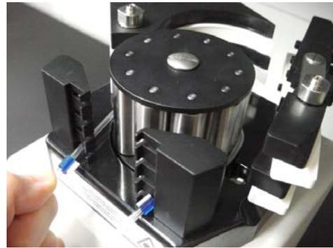
2. Install the tube to the rollers.
