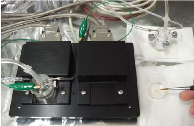
**Figure 3-17.** The 2nd slice is mounted without stopping perfusion to the 1st slice.
