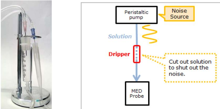
**Figure 3-7.** Inlet/Outlet drippers standing vertically within the dripper stand (left), and how they work to eliminate noise (right).
