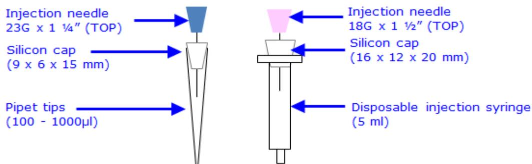
**Figure 4-7.** Specifications for Inlet/outlet drippers.
