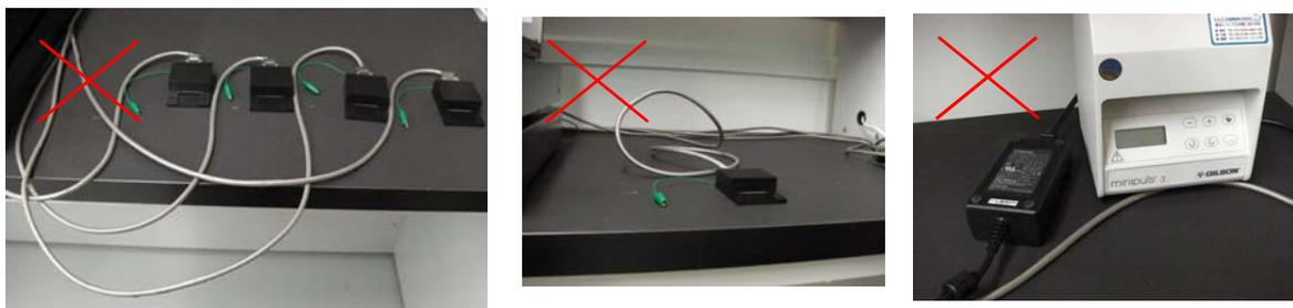
**Figure 2-8.** Bad examples for location of the Connector Cables. Cables are NOT placed flat on the table (left, middle) and touching the peristaltic pump (right).
