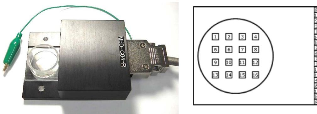
**Figure 2-12.** Type R Connector (left) and electrode orientation when the connector terminal is located on the right.
