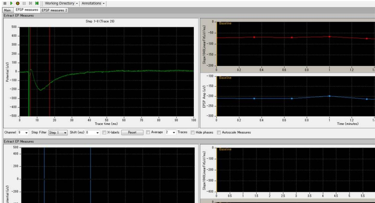
**Figure 6-3.** The [EPSP measures 1-2] tab. Set the cursor for both analyses (red and blue in the right graph) by dragging the cursor in the left waveform chart.
