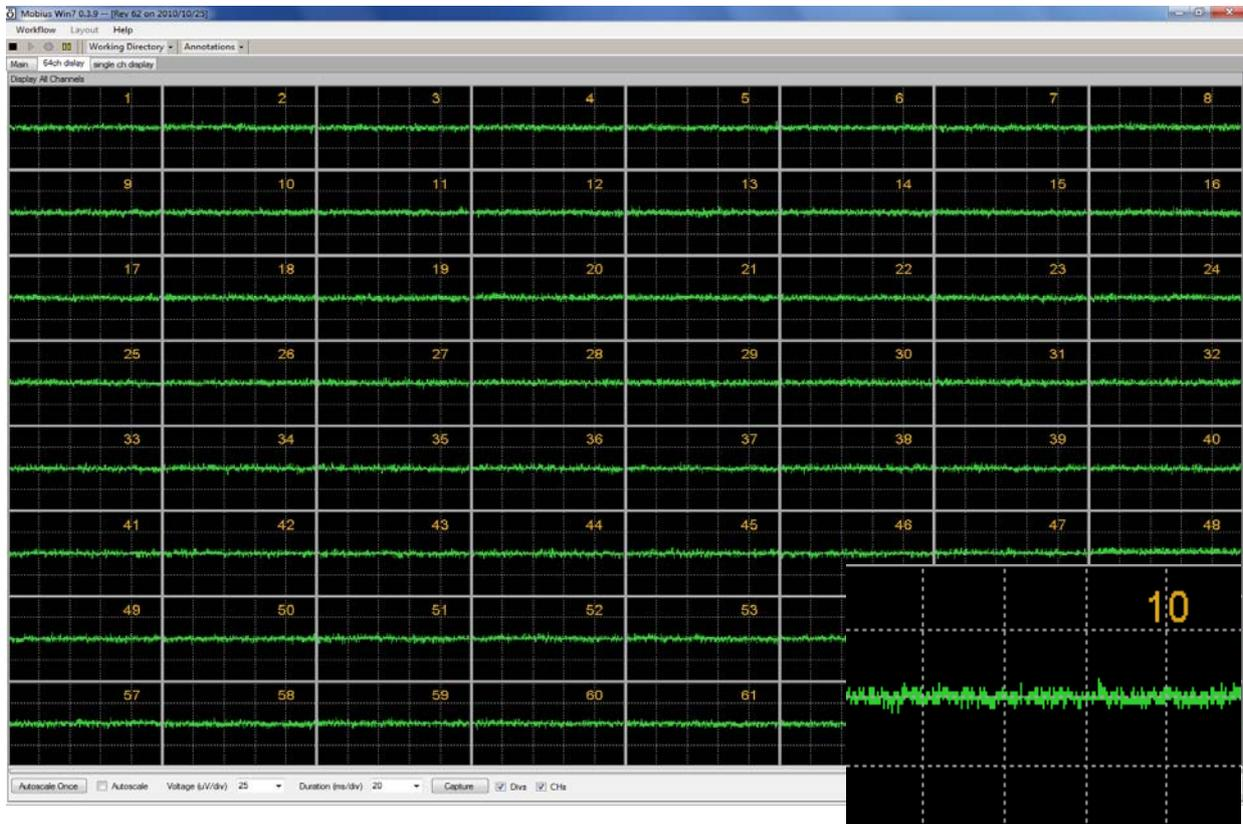
**Figure 2-18.** Appropriate noise level for the MED64-Quad II System ( $25 \mu\text{V}/20 \text{ msec}$ ).
