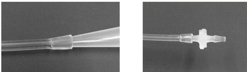
**Figure 4-4.** Making the tube-tip wider first (left), and then connect it to the lure fitting (right).
