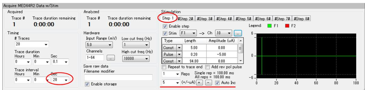
**Figure 6-5.** Acquisition workflow to make I/O curve for Slice 1( Setp1). The stimulation will be applied ONLY to slice 1 (Step 1) with the interval of 20 seconds and stimulus current amplitude will be incremented by 5  $\mu$ A.
