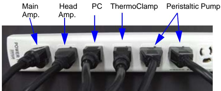
**Figure 3-4.** Grounding the peristaltic pump and ThermoClamp controller through a power supply cord.
