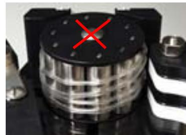
7. Bad example: tubes are not installed horizontally.
