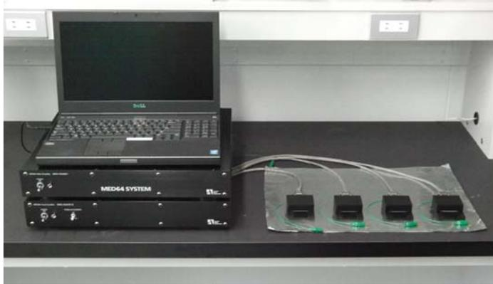
**Figure 2-9.** MED64-Quad II System installed on a lab bench.
