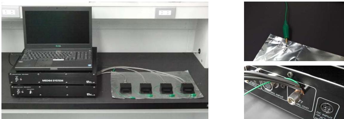
**Figure 2-1.** The MED64-Quad II System installed on a lab bench (left) and grounding the aluminum foil (right).
