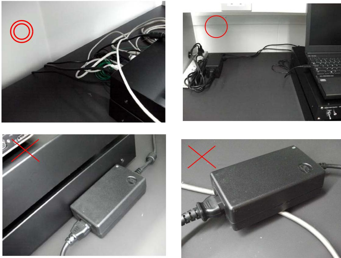
**Figure 2-6.** Examples of good and bad placing for power supply unit.
