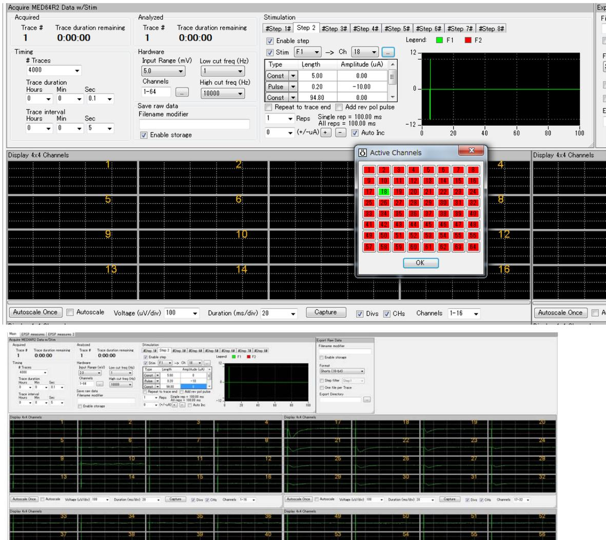
**Figure 6-4.** Looking for the best stimulation channel for the Slice 2 using the Step 2.
