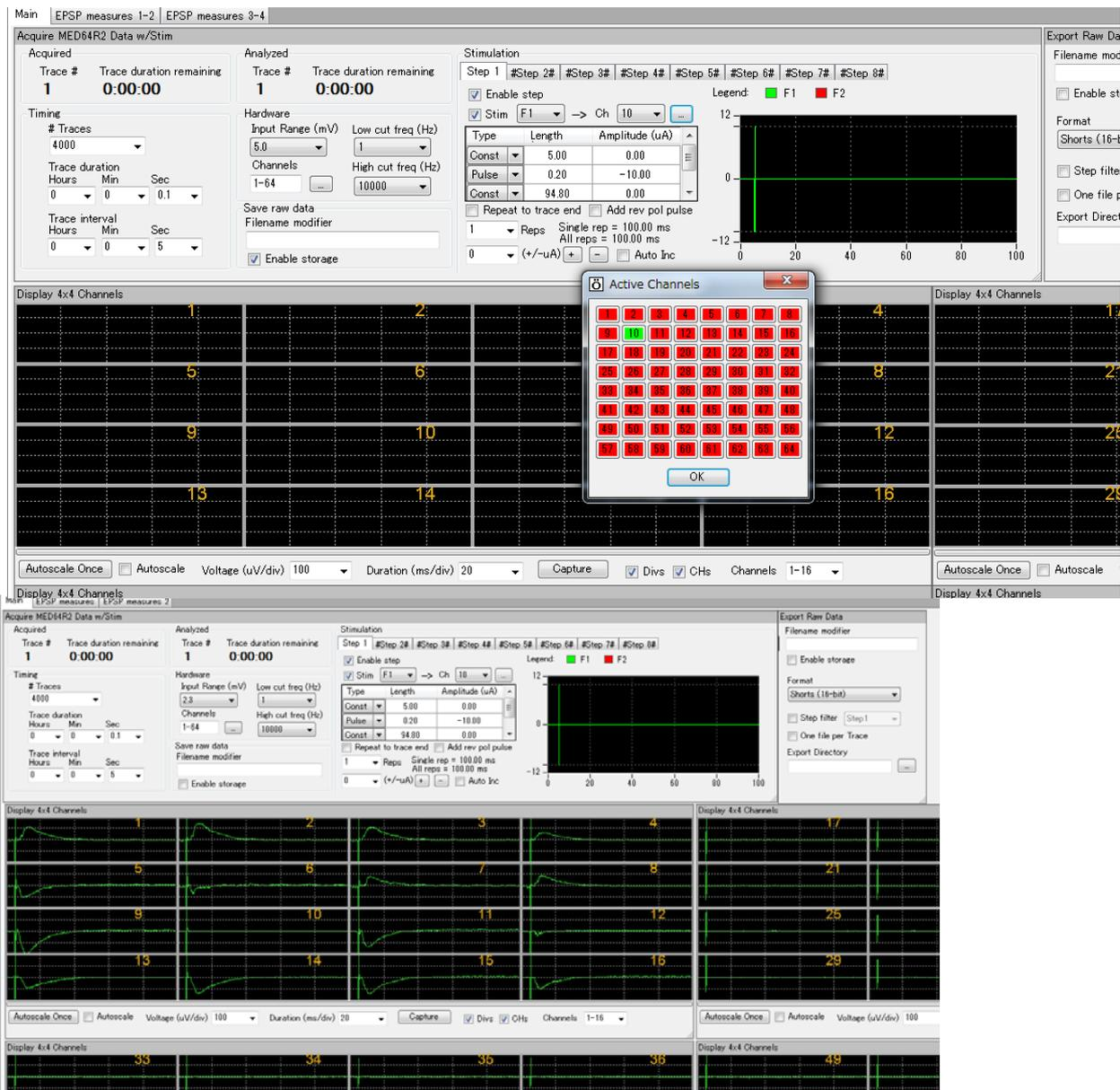
**Figure 6-2.** Looking for the best stimulus channel. Channel 10 is selected for stimulation (top) and stimulation is applied once by clicking the Green button (bottom). fEPSP signals are displayed at the channel 1-9,11-16.
