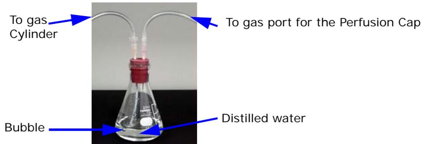
**Figure 3-9.** Moistening mixed gas before sent to the MED Probe.
