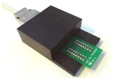
**Figure 2-14.** How to test the MED Mini Connector with the test board.
