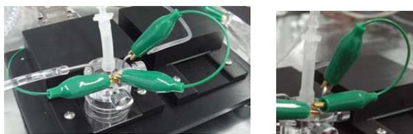
**Figure 3-16.** Grounding the inlet pipe to the ref. electrode.
