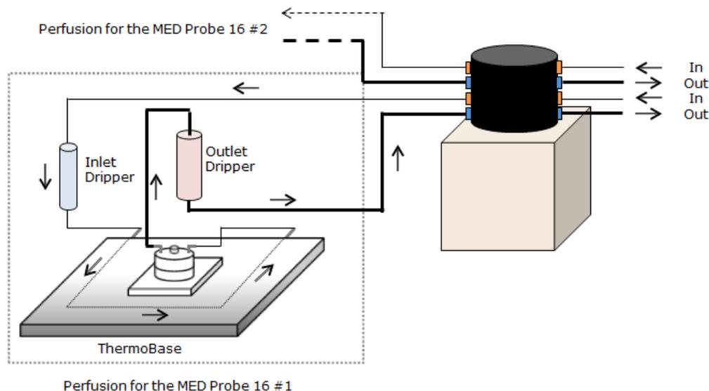
**Figure 3-5.** Perfusion Cap and Tube Kit installed in a peristaltic pump and MED Probe 16.
