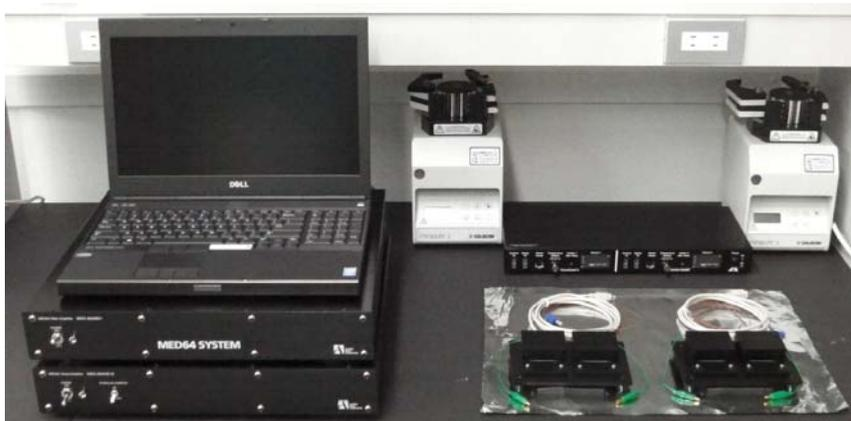
**Figure 2-2.** MED64 Quad II components and perfusion accessories placed on a lab bench.
