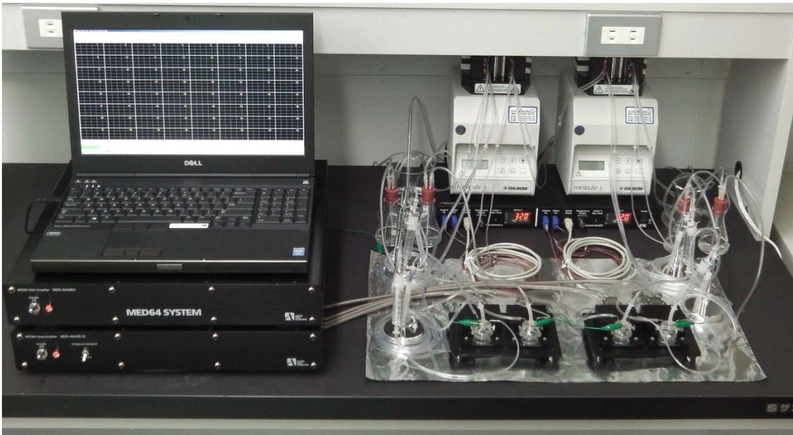
**Figure 3-12.** MED64 Quad II System with perfusion installed on a lab bench.
