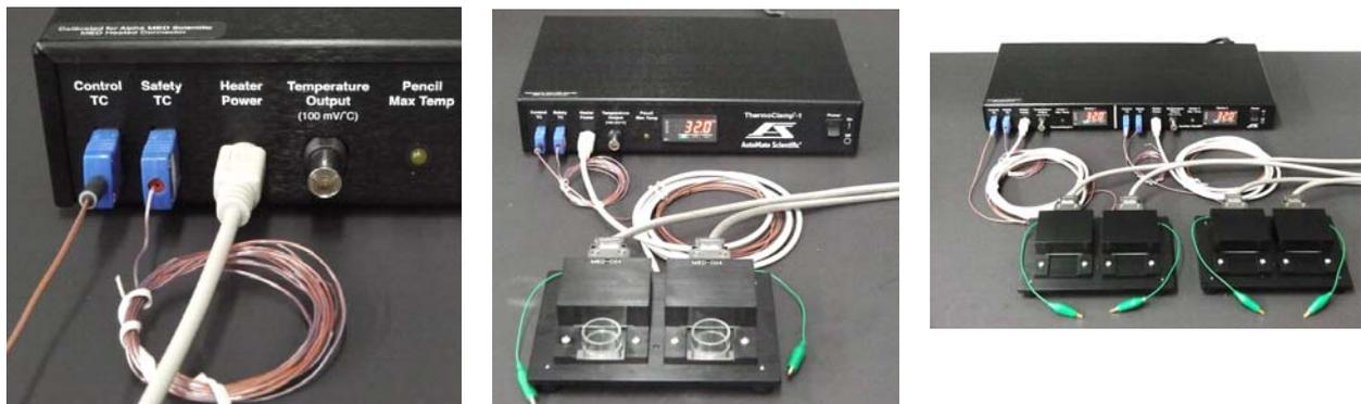
**Figure 2-20.** Cable connections to the ThermoClamp (left), and ThermoBase installed to a ThermoClamp (middle with the ThermoClamp-1, right with the ThermoClamp-2).
