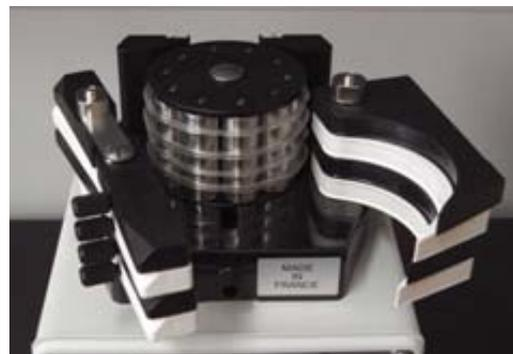
4. Make sure that all tubes are installed horizontally so that they sit under each compression cam.
