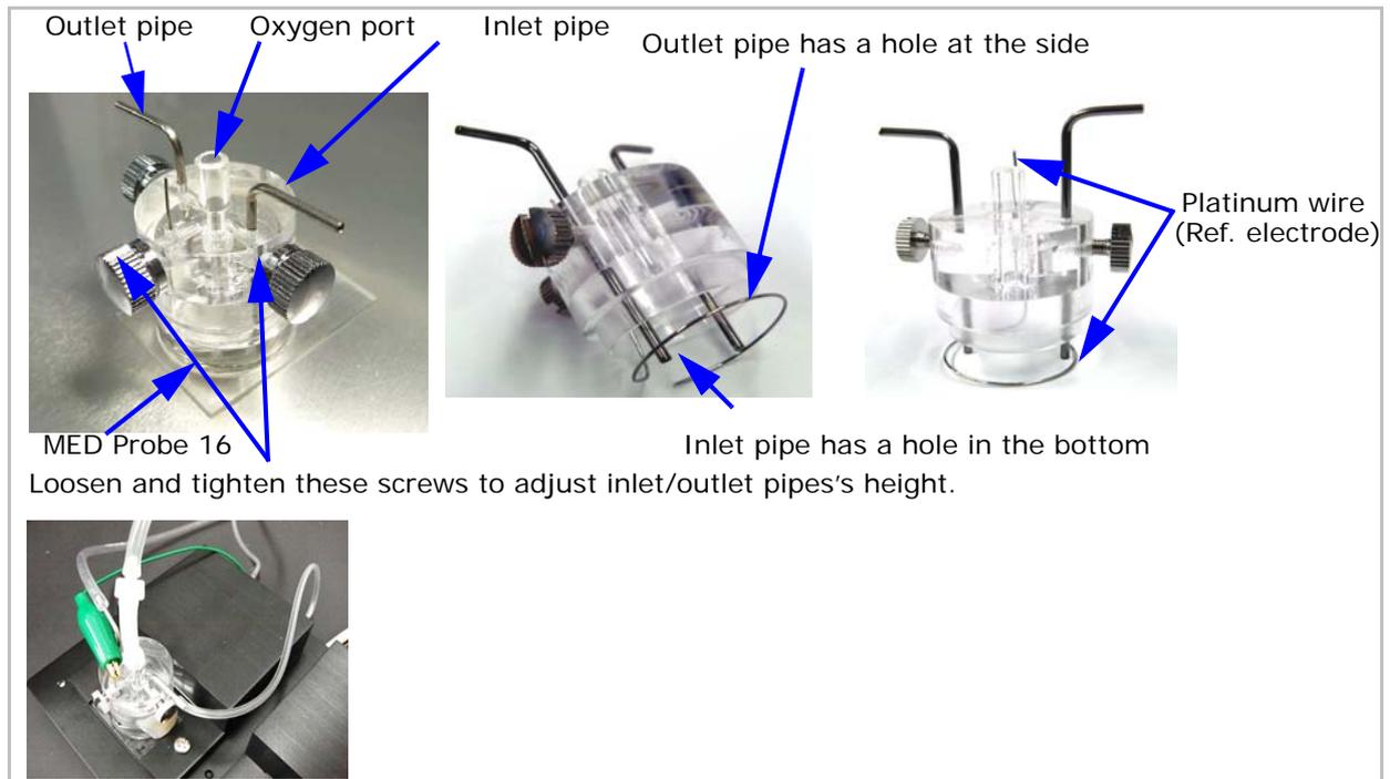
**Figure 3-3.** Perfusion Cap. Details (top) and placed onto the MED Probe 16 (bottom).
