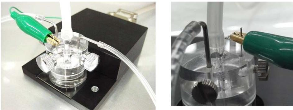
**Figure 3-10.** Grounding the ref. electrode (platinum wire).
