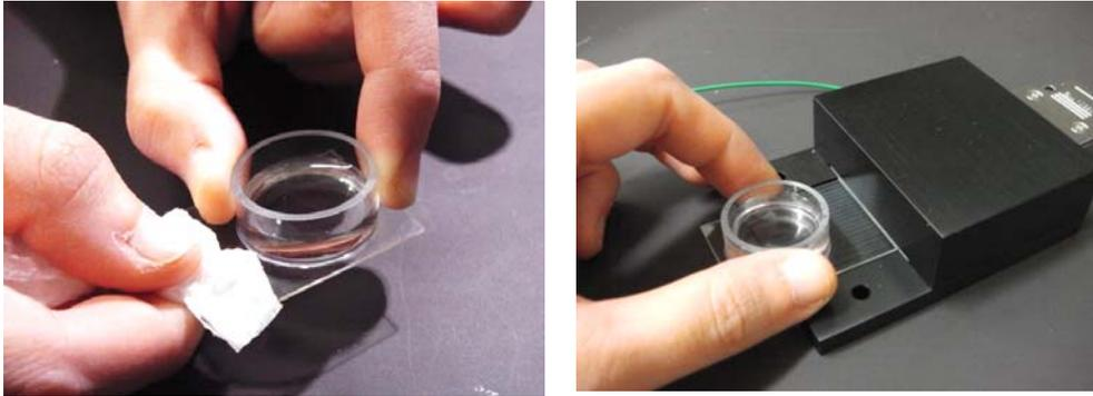
**Figure 2-13.** Loading the MED Probe 16 into the MED-C04 Connector.
