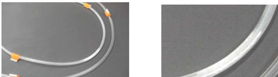
**Figure 4-3.** Examples for the tubing to be replaced due to cracks.
