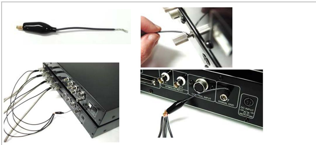
**Figure 2-3.** Grounding the Connector cables to the GND terminal of the MED64 Head Amplifier.
