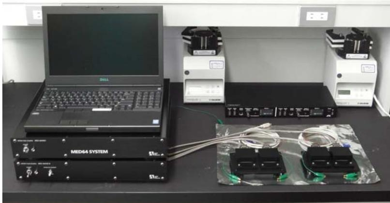
**Figure 2-10.** MED64-Quad II System with perfusion accessories. (Perfusion accessories are not connected yet, and connections will be made in the following section.)
