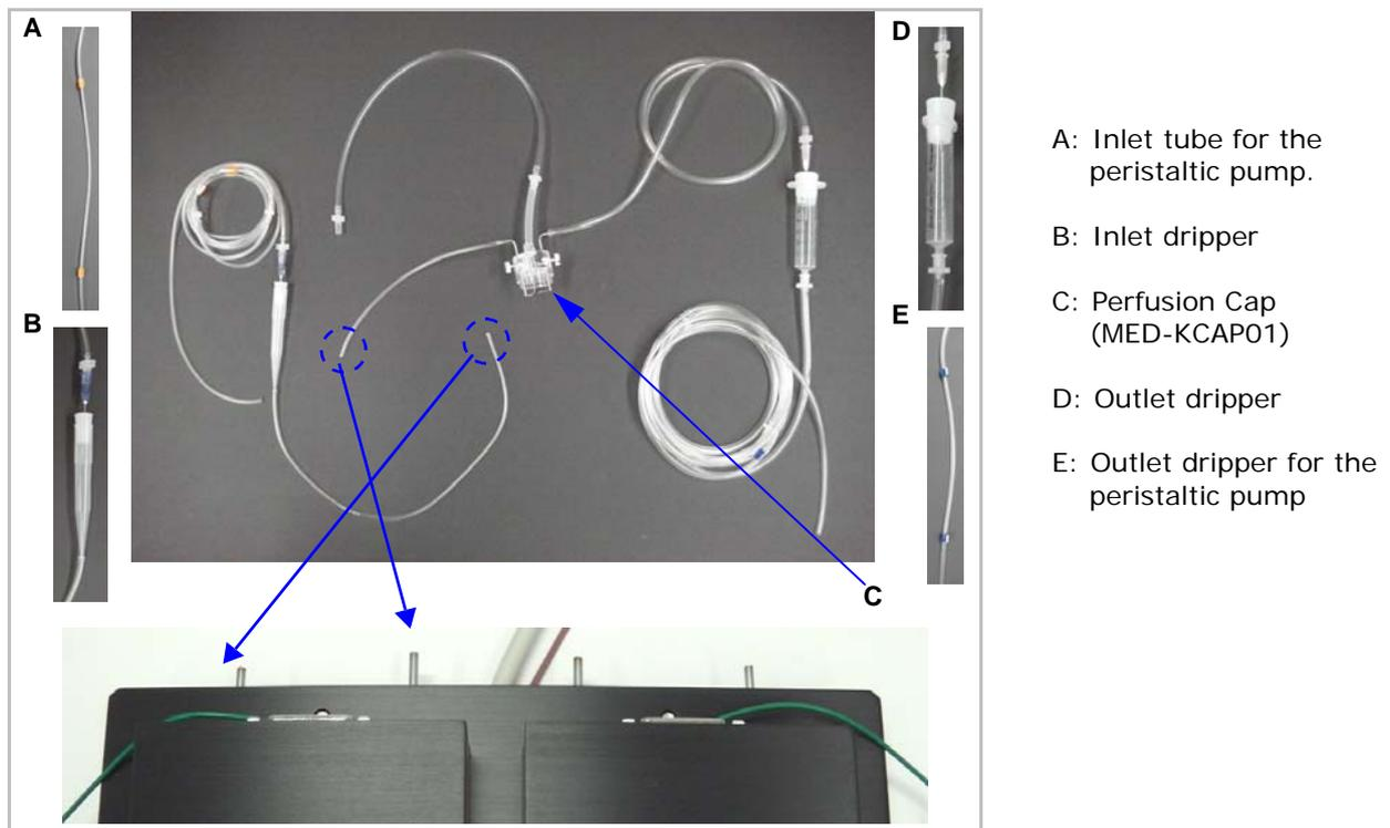
**Figure 3-2.** Perfusion Cap and Tube Kit (top) and perfusion ports in the ThermoBase.
