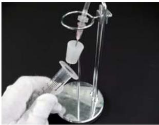
**Figure 3-8.** Installing the outlet dripper to the dripper stand.
