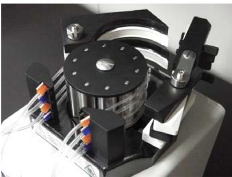
3. Outlet (orange) / Inlet (blue) tubes installed to the Minipuls 3.
