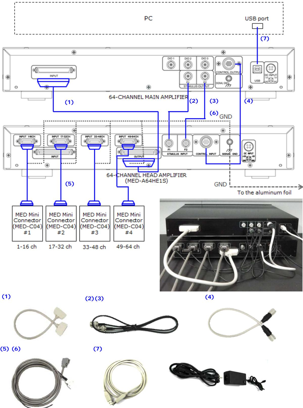
Figure 2-4. Cable connections for the MED64-Quad II System.
