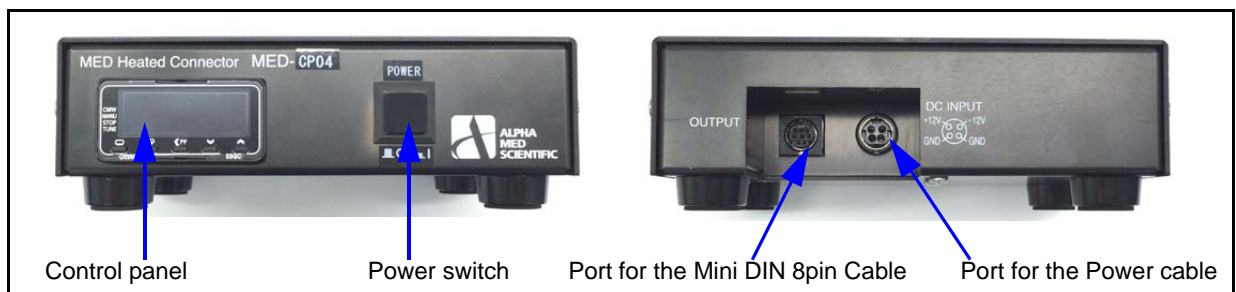
Figure 3. Temperature controller. Front view (left) and back view (right).
