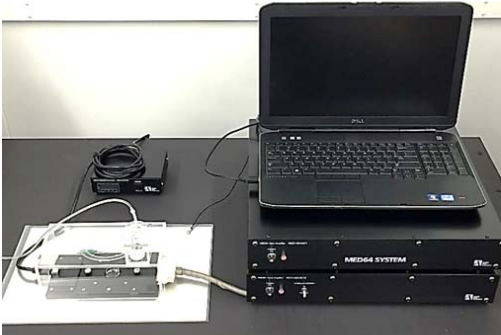
Figure 7. The MED64-Basic System with the Connector Cover installed on a lab bench.
