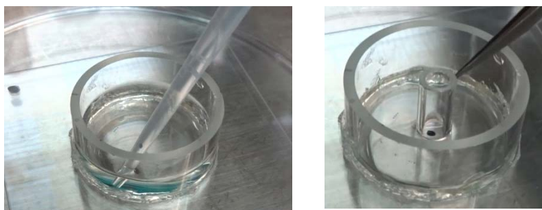
Figure 3. Removing the SureBond (left) and Placing cloning ring around the electrodes (right).
